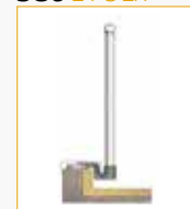
Insulated parapet EVOZx
